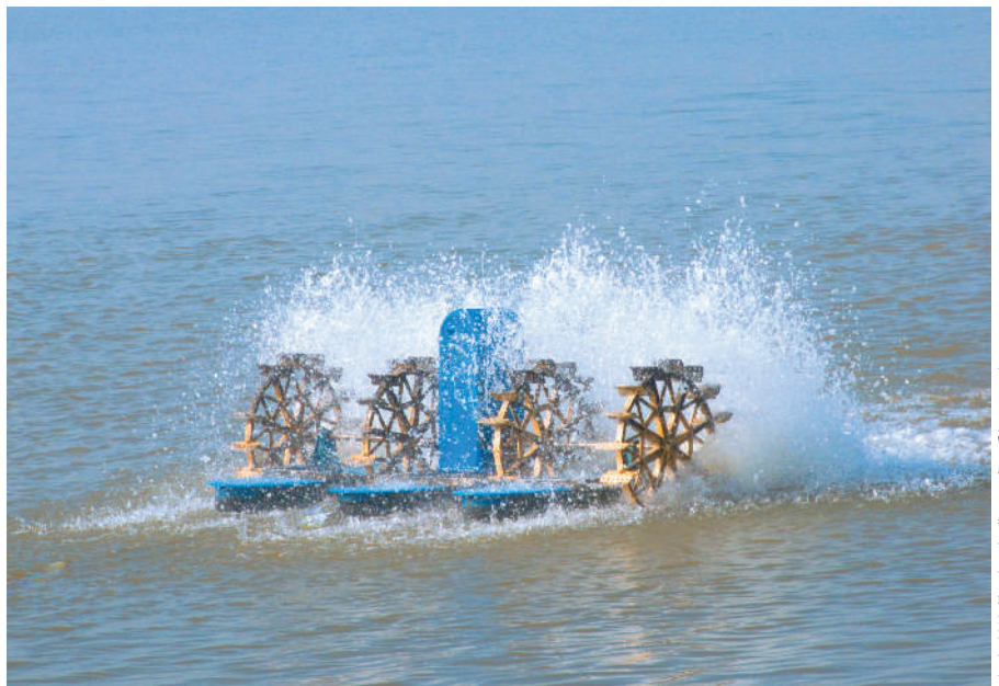
FIGURE 13-21 Portable paddlewheel aerators can be powered by a tractor PTO, mounted engine, or an electric motor.
