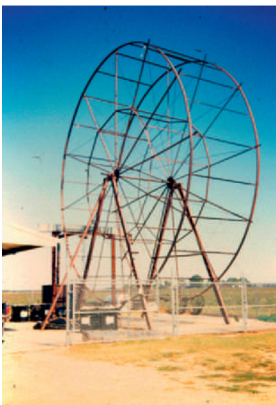
FIGURE 13-25 After seines are made, they must be treated so that they do not rot in water. This “ferris wheel” is used to wrap the treated seine around while it dries.
