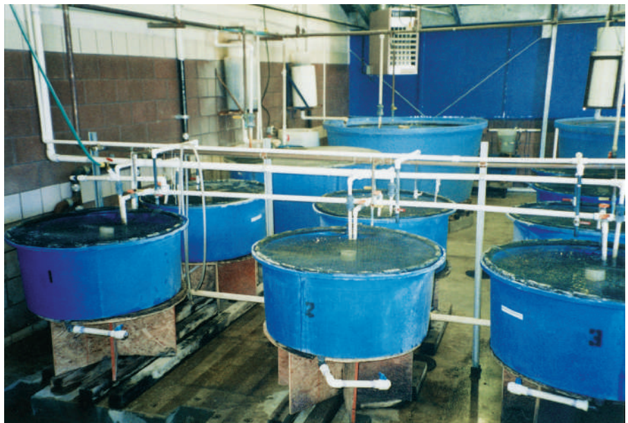
FIGURE 13-15 Circular fiberglass tank being used in a recirculating system at a high school.
