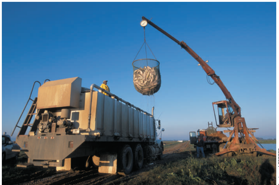
FIGURE 13-27 Boom mounted brailer lowered to live haul truck during loading of catfish.
