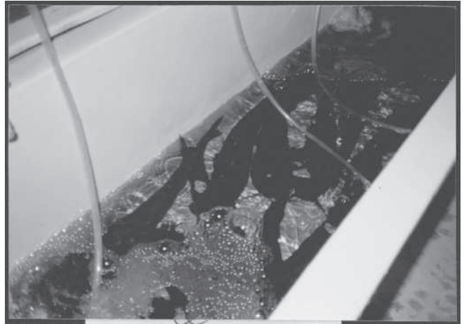
FIGURE 13-24 Small diffused air system being used to maintain catfish in a small laboratory tank.
