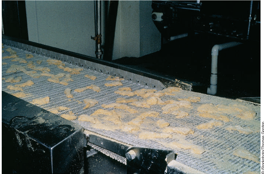
Figure 3-14 Fillets are quick-frozen on a spiral freezer or a tunnel-type freezer.
