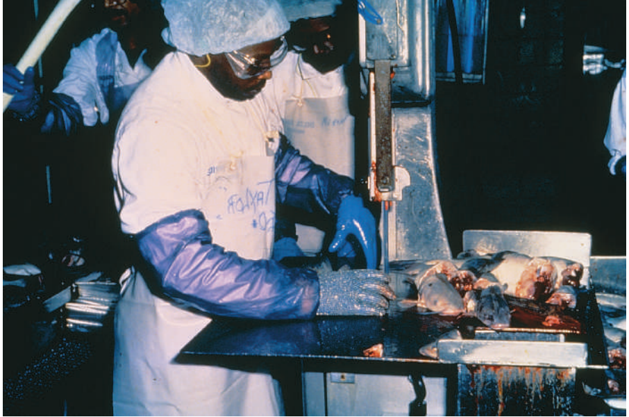
Figure 3-12 Deheading channel catfish with a bandsaw.
