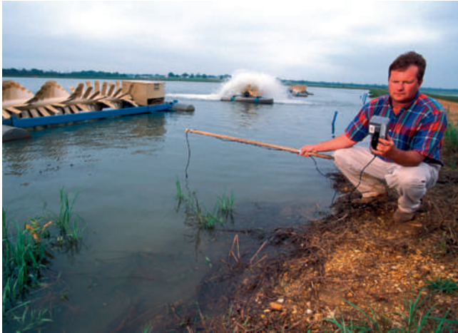
FIGURE 13-23 Scientist taking an oxygen reading on a pond with brush aerators anchored in the background.
